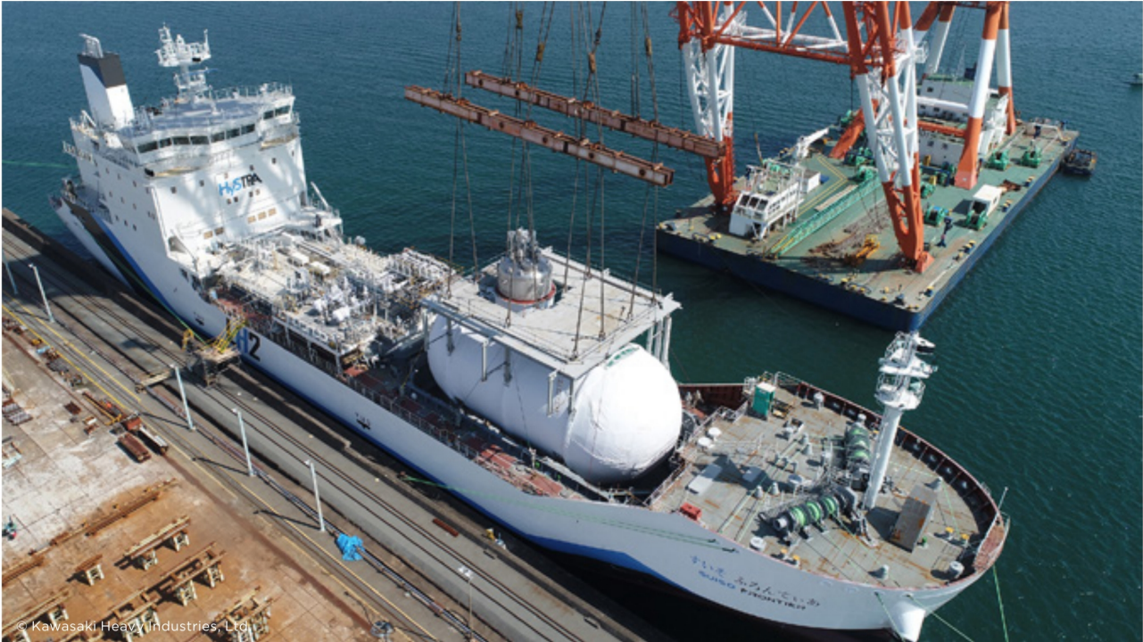
Figure 15: The Suiso Frontier is the First Liquid Hydrogen Carrier, Launched in 2021 and Intended for Use in the HESC
